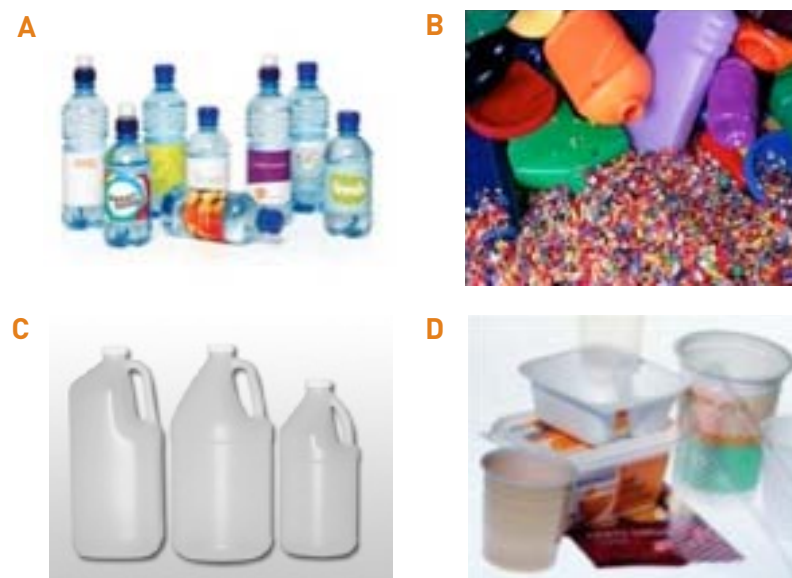
Figure 10 Examples of different commonly used plastic polymers and their products. A. Clear PET used for mineral water; B. Coloured PET used for common household products; C. HDPE natural used for milk containers; and D. mixed plastic packaging consisting of various plastic polymers
