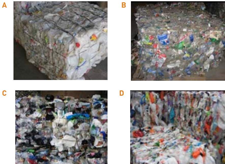
Figure 11 Examples of different MRF outputs. A. HDPE Natural; B. Clear PET; C. rigid household plastic packaging; and D. plastic film 21
